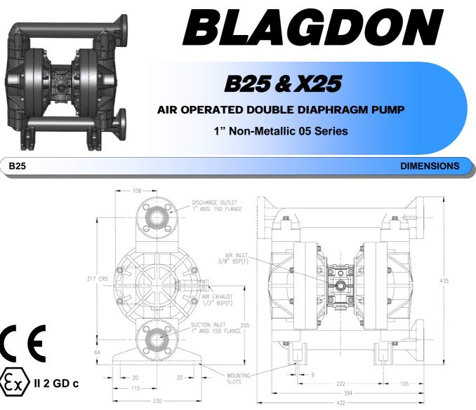
General Assembly :- B2505 Moulded Pump, all dimensions +/- 3mm
