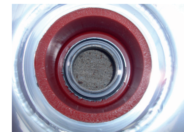
Coating in seal chamber for increased wear resistance.
